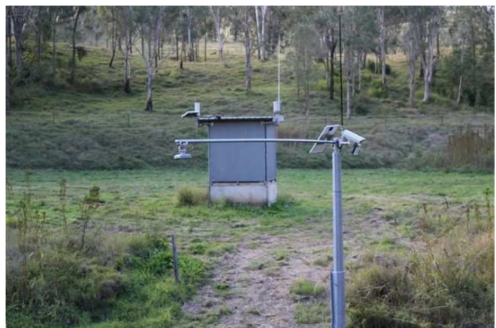
New vs Old - Radar FEWS with existing water data logger Hut in the background.
