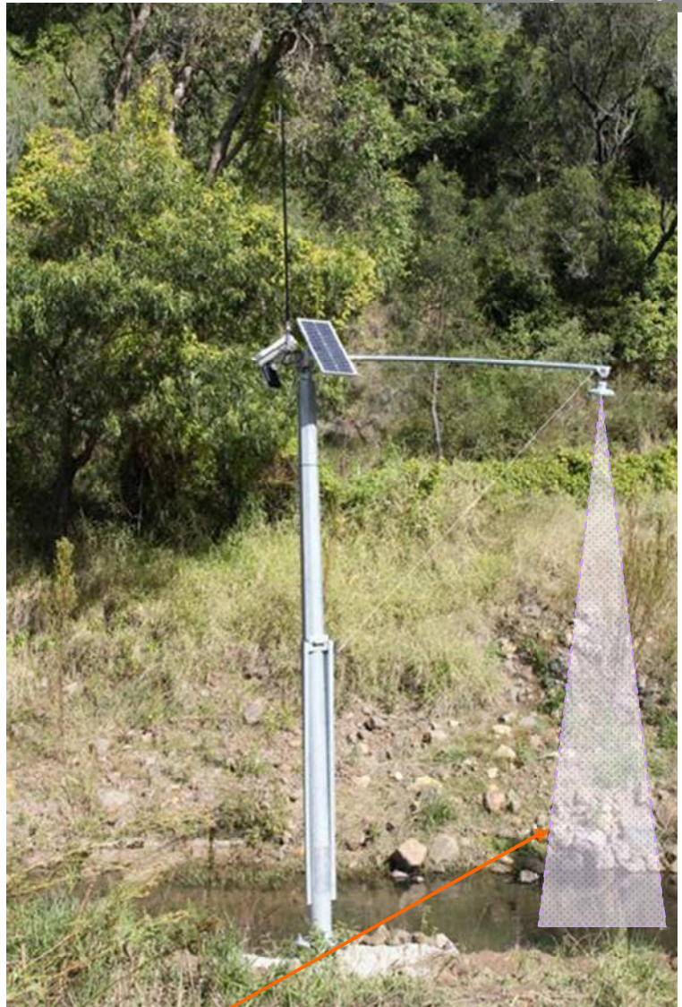
Radar Sensor detects water levels with 3mm accuracy!
